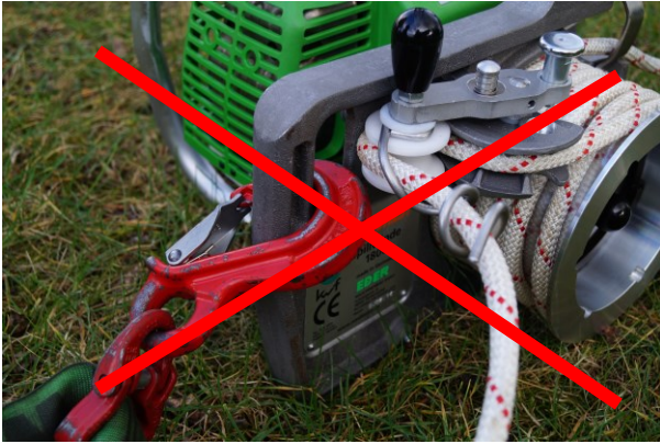
Fig. 7: wrong fastening the EDER Powerwinch 1800
