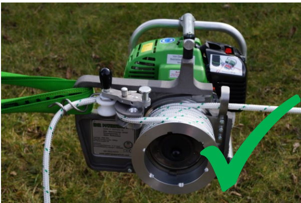
Fig. 8: Correct fastening the EDER Powerwinch 1800
