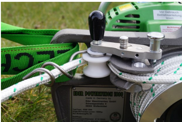
Fig. 6: Guiding the rope through the clamp and the spring wire
