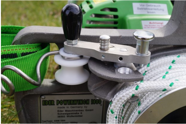
Fig. 4: Guiding the rope through the clamp
